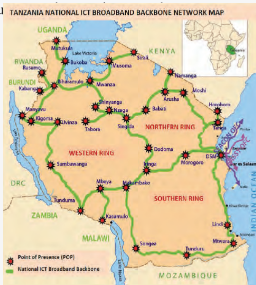
The National fiber ICT Broadband Backbone provides international links to Tanzania's landlocked neighbours, namely; Uganda, Rwanda, Burundi, DRC, Zambia and Malawi.
